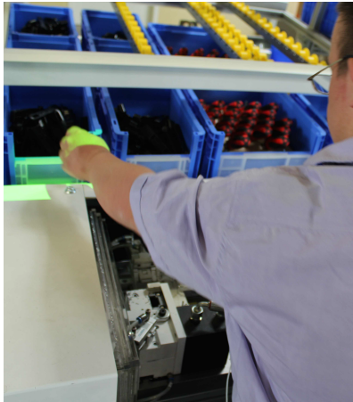
Figure 3: Assistance by lighting that indicates the correct box to pick from for an assembly task, which is useful for people with severe cognitive decline, but too boring for people with just minor cognitive impairments [8]
